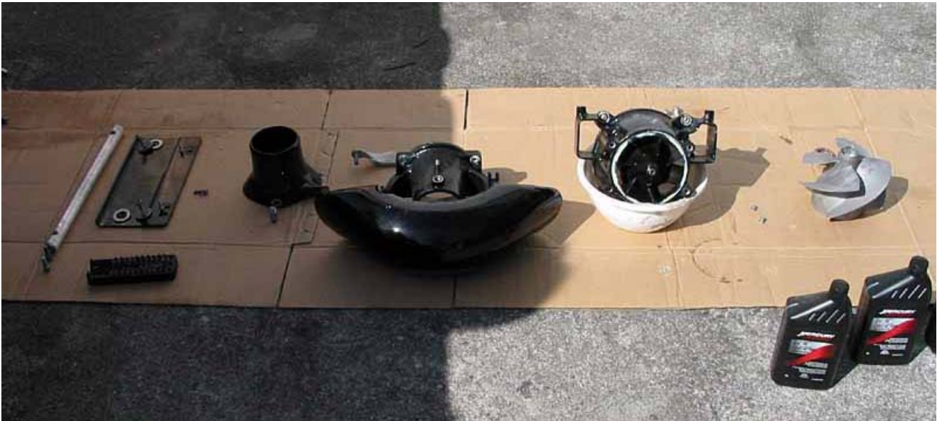
Picture 7: Lay out all parts that you remove in the order you removed and together with the nuts and bolts that go with them. This will make reassembly much more efficient.
