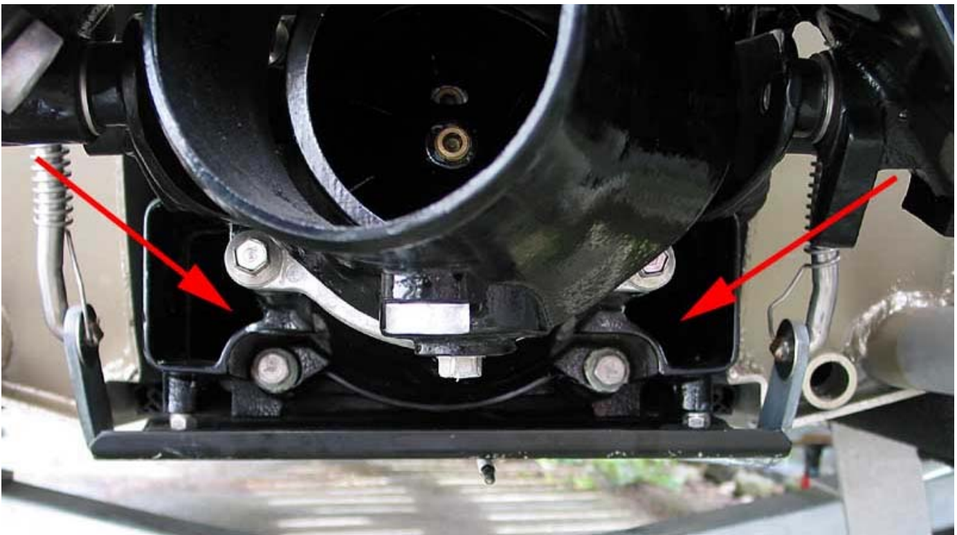
Picture 5: Spray WD40 or penetrating oil where indicated.
