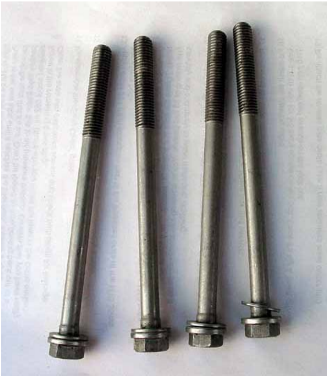
The bolts cleaned and wire brushed.
