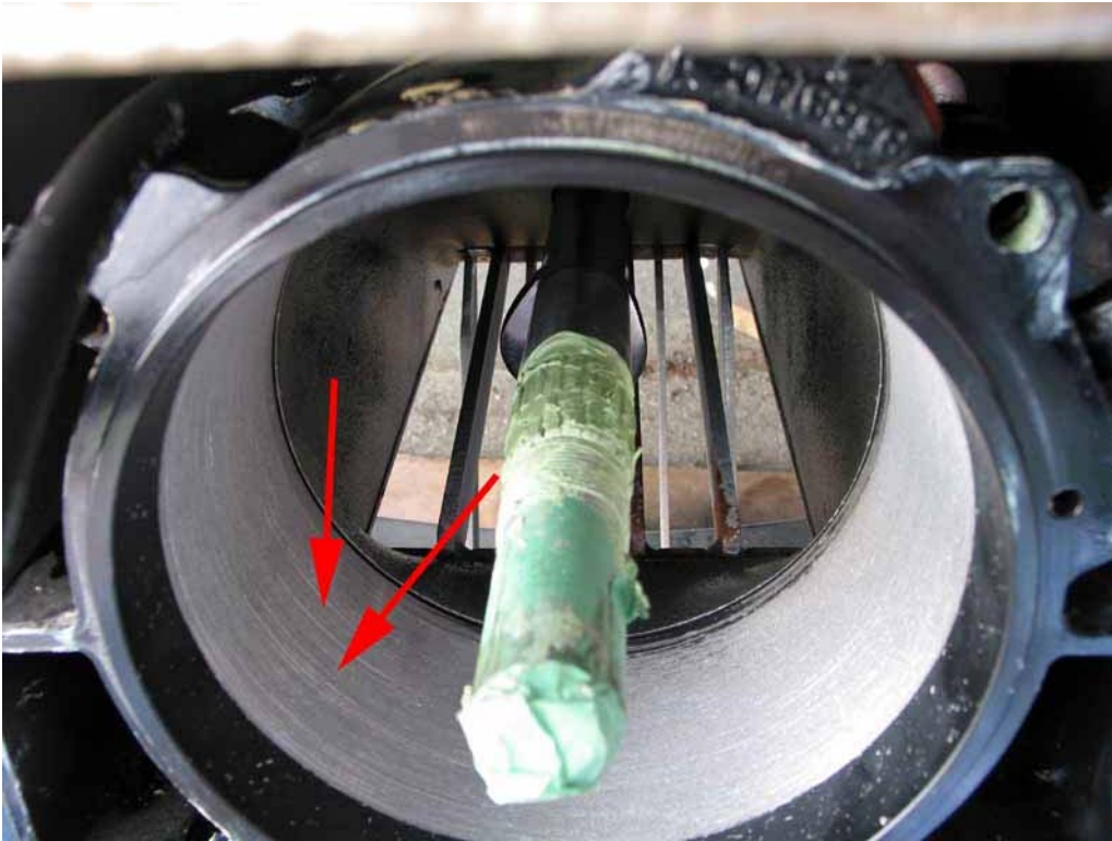
29. Inspect the wear ring for gouges and other damage. If the damage is too great, replace the wear ring or have a Stainless Steel insert made.
